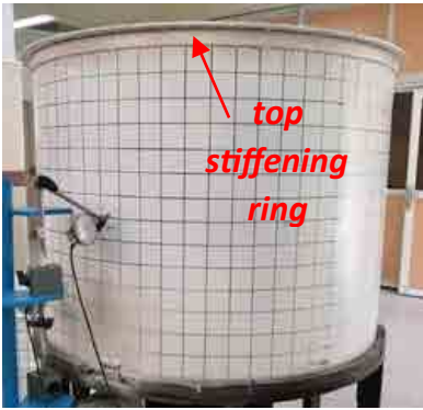
Fig.1. Steel thin-walled open-top tanks
