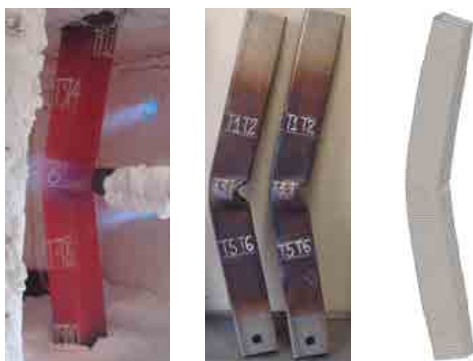
Figure 1. (a) Fire bending test of stainless steel RHS members and (b) corresponding numerical simulations [1]
